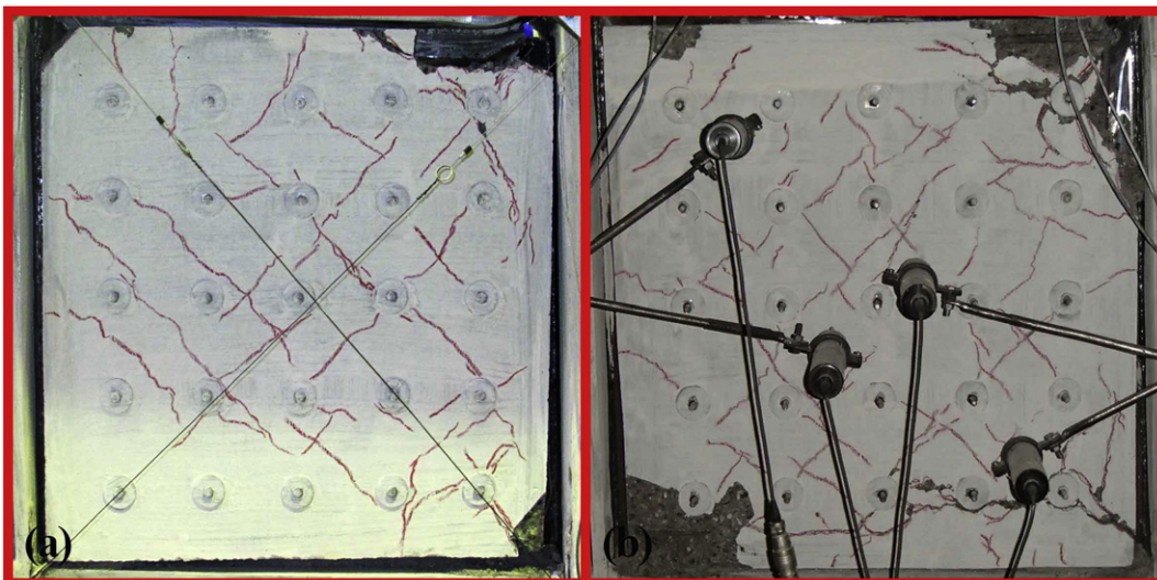
Fig. 13. Specimen C-SPSW-DL after the test: (a) front light-weight panel (b) back light-weight panel.
