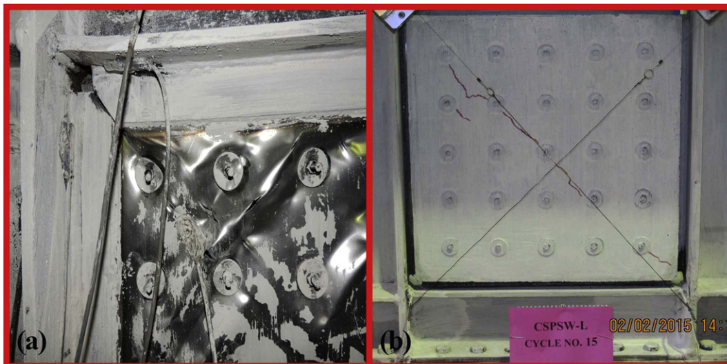
Fig. 9. Specimen C-SPSW-L: (a) the fracture of the steel plate in the corner (b) initial diagonal hairy cracks.
